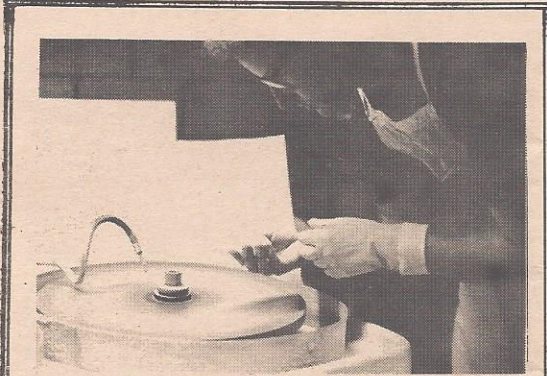
Drew Tousley takes a look at the shaped crystal to determine what additional shaping may be necessary before it is moved to the polishing unit.
